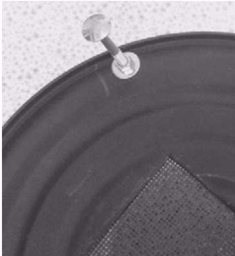
Photo 2: The dryer from underneath. The picture shows one of the support screws and the centred mosquito mesh.
