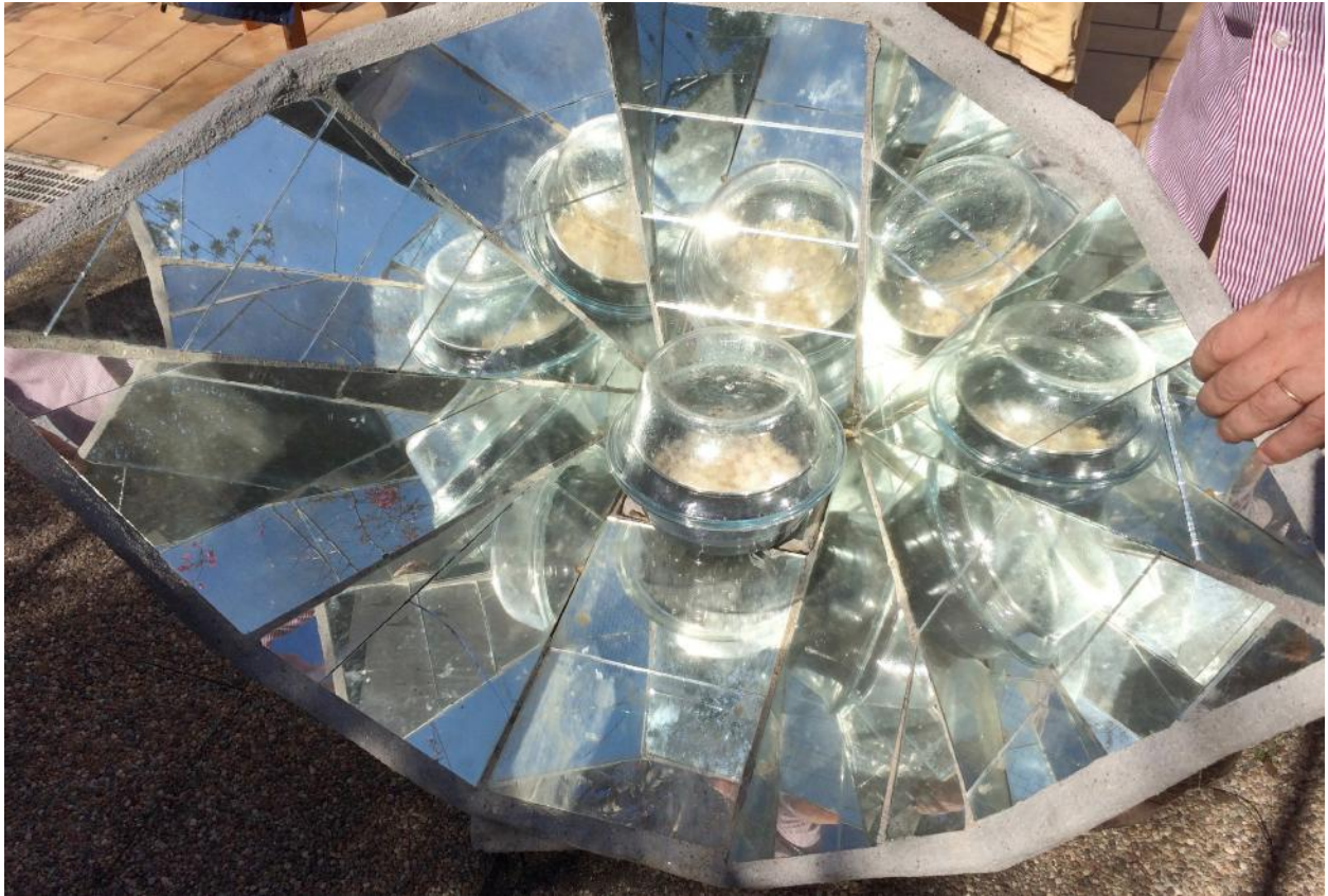
Photo 2: The funnel cooker "Pucca" made of concrete by Celestino Ruivo, Portugal, It can be left outside throughout the year. A weight of 80 kg protects these models from theft.
